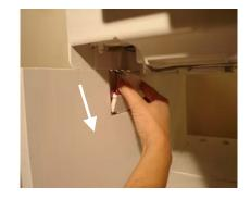
B Disconnect the reed switch carefully and connect the new reed switch.
