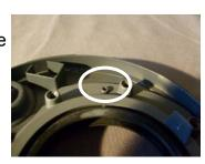
Note: when placing the retainer please make sure that the white pin is situated on the dot on mechanism.
