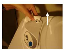
Remove the control panel.
