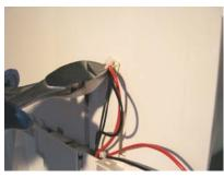
Remove reed switch housing by Н pressing both lips on the side.
