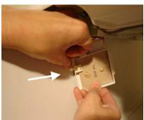
Place the new reed switch back into the toilet and place waste tank back into the toilet.
