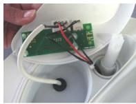
Cut the tyrap and release connector by pressing lip on connector housing.
