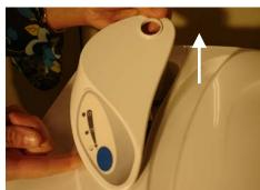
Remove the control panel.
