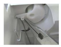
Remove 3 screws from pivotting bracket, and remove bracket.
